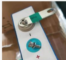
M4 Screws And Busbar
